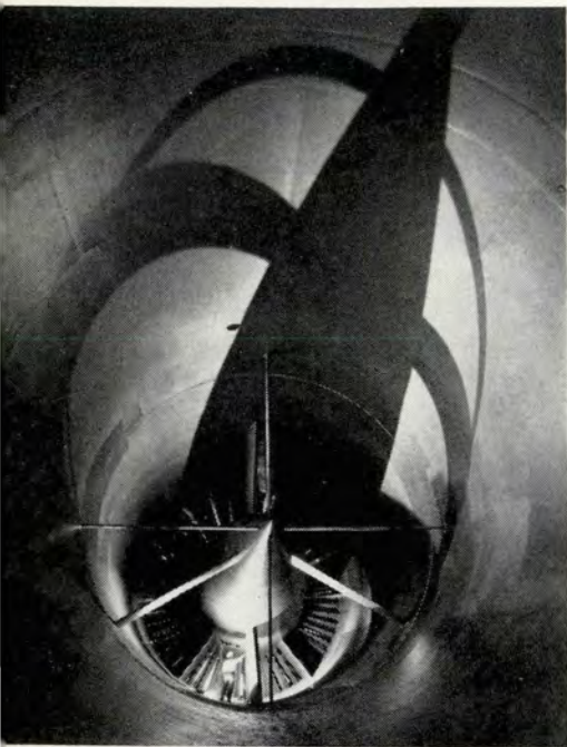
Compressor to power and spraybars to cool airflows, 0.5 to 1.5 Mach.
